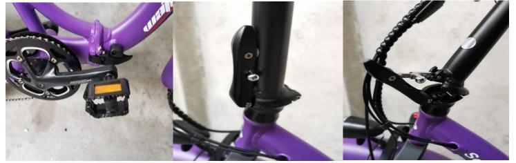
3<sup>rd</sup> – Lift up the small black latch where the folding bracket is located on the main frame. Then pull towards you the main black latch to unlock. When folding make sure the pedals are in roughly the same position as the photo
