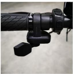
When using the throttle from a standing start please ensure you start in low PAS. Starting the bike in a high PAS and the highest gear can put a lot of stress on the motor and will wear the motor faster.
