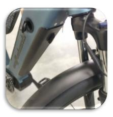
To remove the battery, turn the wheel slightly so you have better access to battery. Turn the key to the unlock position and then turn the lever on the battery case to release the battery
