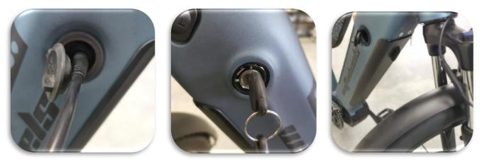
To remove the battery, turn the wheel slightly so you have better access to battery. Turn the key to the unlock position and then turn the lever on the battery case to release the battery
