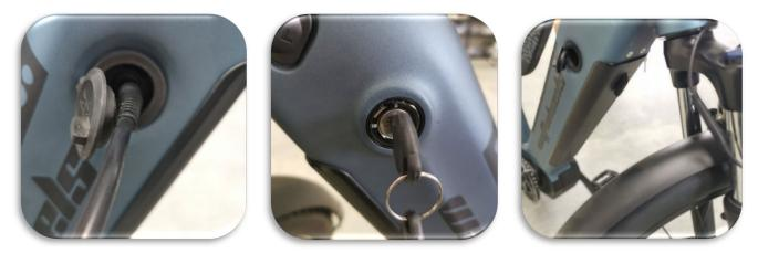
To remove the battery, turn the wheel slightly so you have better access to battery. Turn the key to the unlock position and then turn the lever on the battery case to release the battery. Note on the low step frames the battery is removed from the top.
