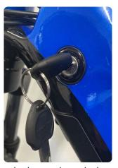
To remove the battery, turn the wheel slightly so you have better access to battery. Turn the key to the unlock position and then turn the lever on the battery case to release the battery
