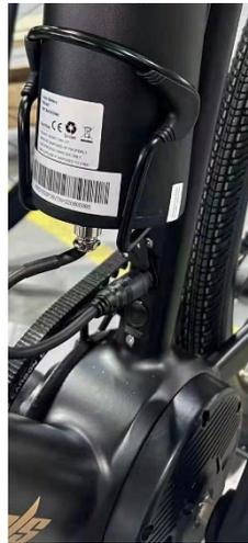
The charge left in the battery should be 50%-75% if storing for long periods of time (two months or longer). Periodically check the charge of the battery
