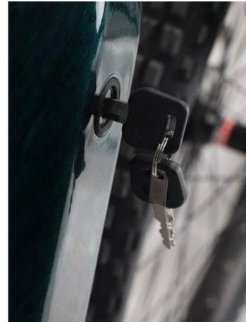
To remove the battery, turn the wheel slightly so you have better access to battery. Turn the key to the unlock position and then turn the lever on the battery case to release the battery.
