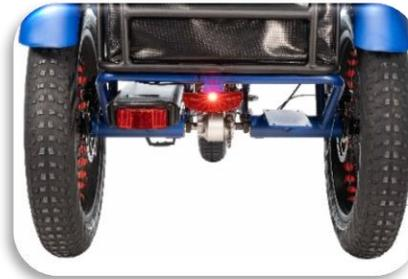
To remove the battery, Turn the key to the unlock position and then slide the battery out of the battery holder. Removing the battery from the trike when storing it for a long period of time is recommended. In this case store it in a cool, dry area away from water. The charge left in the battery should be 50%-75% for long storage times. Cleaning the battery and battery housing should only be done while disconnected and powered off. Use a dry rag or if needed a lightly damp rag.
