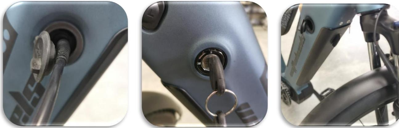
To remove the battery, turn the wheel slightly so you have better access to battery. Turn the key to the unlock position and then turn the lever on the battery case to release the battery
