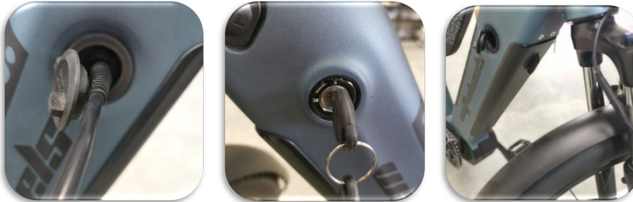
To remove the battery, turn the wheel slightly so you have better access to battery. Turn the key to the unlock position and then turn the lever on the battery case to release the battery. Note on the low step frames the battery is removed from the top.
